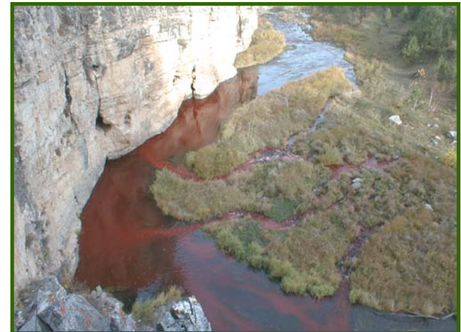
Top: Gravel Springs, Black Hills of South Dakota, prior to dye arrival; Bottom: Gravel Springs at 69 minutes after dye tracer released in Box Elder Creek (Photos by Derric L. Iles)
