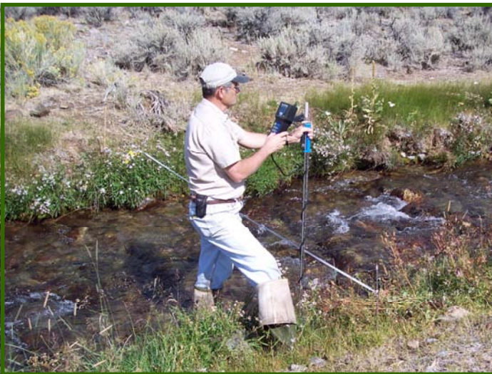
Robert Whittier taking flow measurements in the Pahsimeroi
