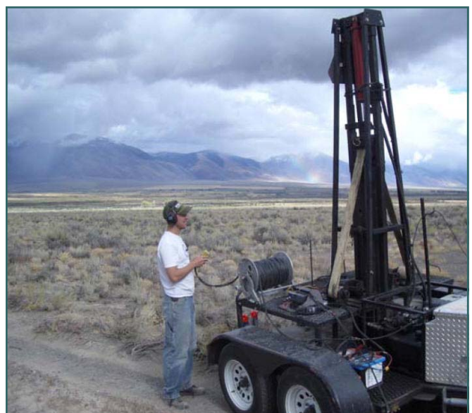
Seismic trailer generating a sound pulse to measure density of underlying geology.
